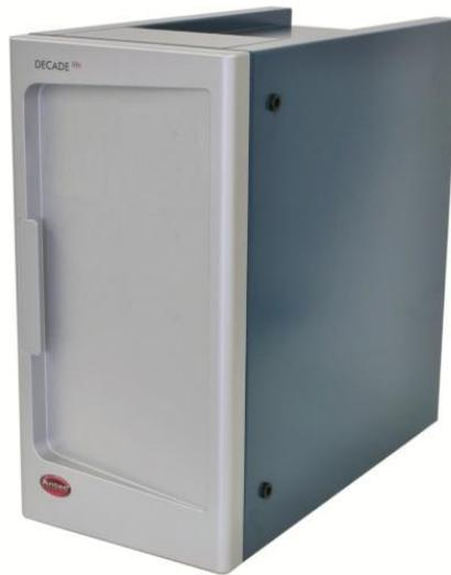
The **DECADE Lite** has the same performance as the famous DECADE Elite. It has an integrated oven with Faraday cage, it is equipped with the superior ADF and has control for one flow cell (*single cell control*). The DECADE Lite has *DC mode only* and is operated by PC control software (free). The DECADE Lite is compatible with all Antec flow cells.
